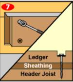
8. Now that the ledger is securely in place, take silicone caulk and fill in the holes with the lag bolts. Then run a bead of caulk along the seam between the siding and drip edge above the ledger.
